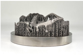
5 Partials / CoCr / built in 3.5h
