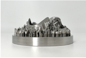
Mixplate (Crowns, Bridges and Partials) / CoCr / built in 3.5h
