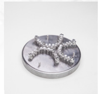
3 abutments in CoCr built in 3.20 h Post processing: connectors milling
